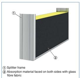
The splitters have a mineral wool infill as absorption material.
