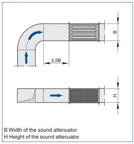
Horizontal installation only for splitters up to height 1200 mm
