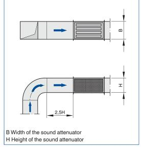
Horizontal installation only for splitters up to height 1200 mm
