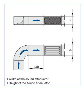
Upstream conditions after bends, junctions or a narrowing or widening of the duct, horizontal upstream section, splitters horizontal
