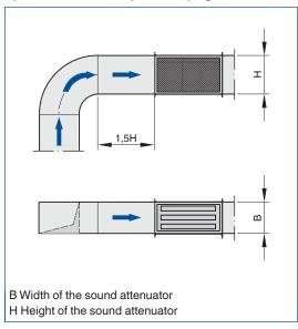
Upstream conditions after bends, junctions or a narrowing or widening of the duct, vertical upstream section, splitters horizontal
