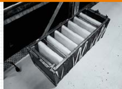
Cumbersome and time-consuming filter changes: The filter elements had to be manually folded into the steel boxes.
