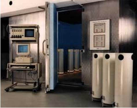
This facility is used for the standardised identification of the cooling capacity of passive water cooling systems according to standards DIN EN 14240, 14518 and 15116. This is where new developments are advanced, catalogue data determined and measurements are taken as proof of performance for major projects according to customer wishes.
