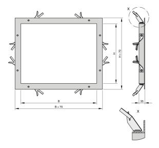
Before the subframe is mortared in, the fixing tabs must be bent and spread (by others).
