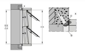
① Threaded stud Installation subframe ③ Fixing tab
