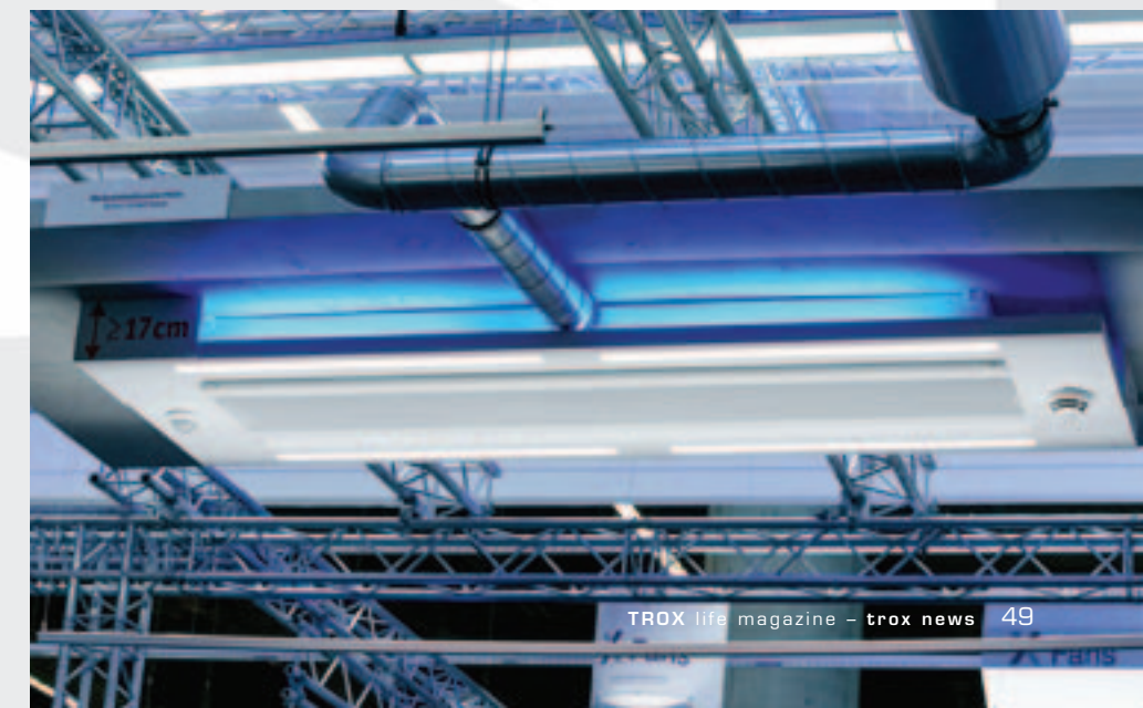
The DID 642 active chilled beam is impressive because of its slim construction. The new nozzles cause fewer pressure losses and allow for a broader range of applications. The unit can be installed freely suspended, in plasterboard ceilings or in open cell ceilings.
