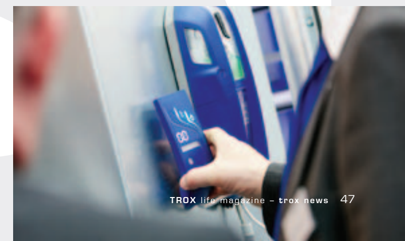
Handy: The mobile display and control panel for the RM-O-M duct smoke detector.
