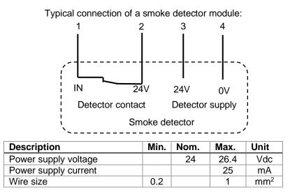
All Easy3-B230 are delivered with a wire connecting pins 1 and 2 to simulate a smoke detector.
