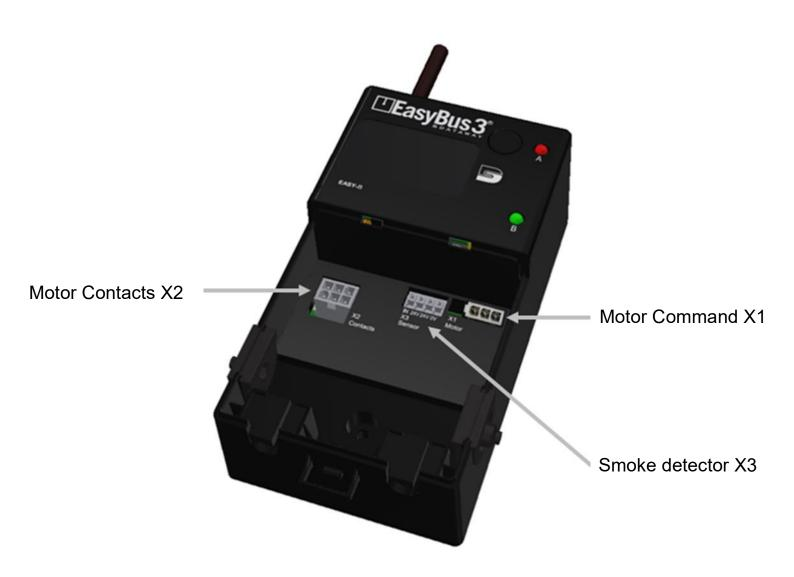
The motor command and motor contacts connectors are compatible with <u>Mate-N-Lok</u> connector type. The matching type must be assembled on the fire damper motor cables to ensure proper connection.
