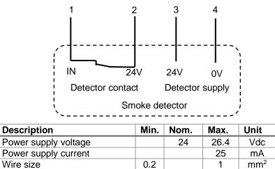
All Easy3-B24 are delivered with a wire connecting pins 1 and 2 to simulate a smoke detector.
